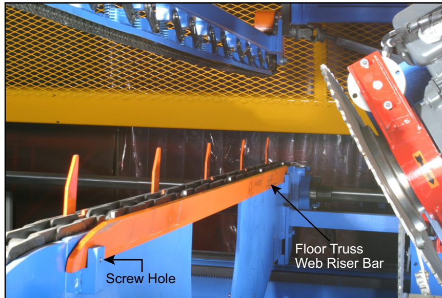
Figure 3-13: Attaching the Floor Truss Web Riser Bars
