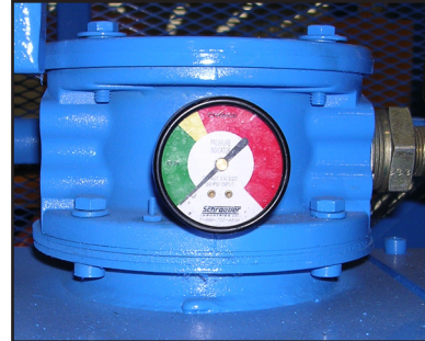
Figure 7-5: Cooling Circuit Filter
