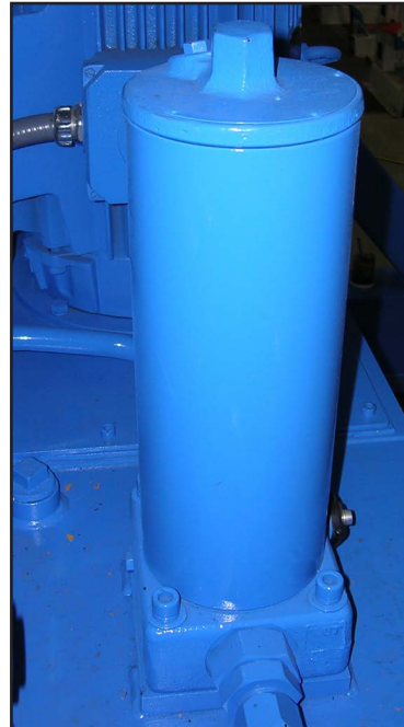
Figure 7-6: Power Circuit Filter
