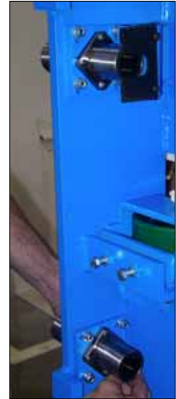
Figure 4: Attach Bearing Mount Plates
