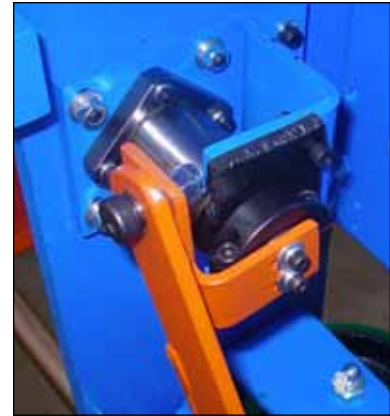
Figure 6: Attach Dog-Leg Assembly to Bumper Shaft
