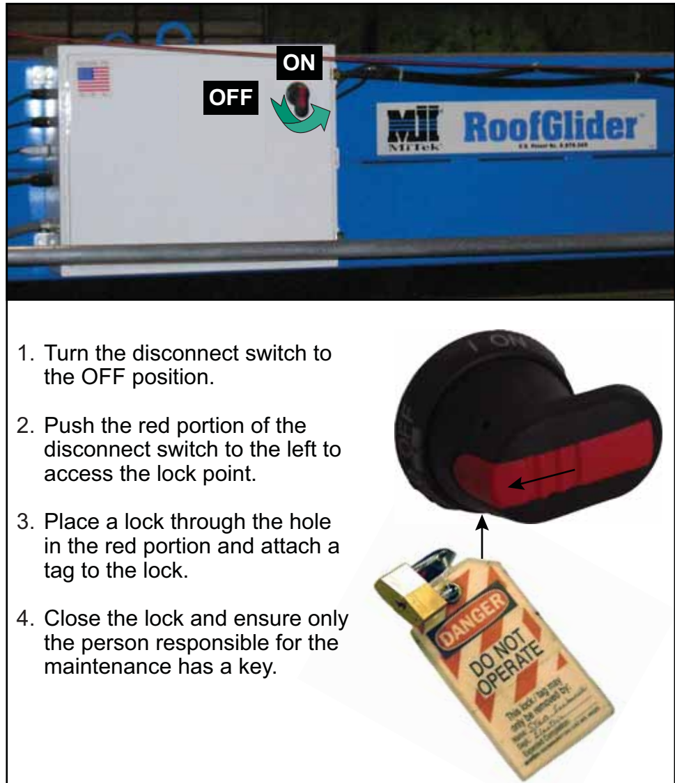
Figure 2: How to Lockout/Tagout
