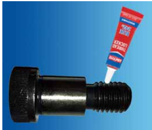
Figure 9: Apply Loctite to the Shoulder Bolt Threads
