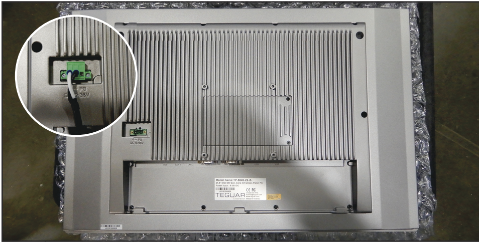
Figure 4: Placing Terminal Block on the Computer
