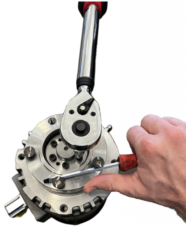
Figure 6: Holding the Hub Still (motor / hub shown outside saw chamber)
